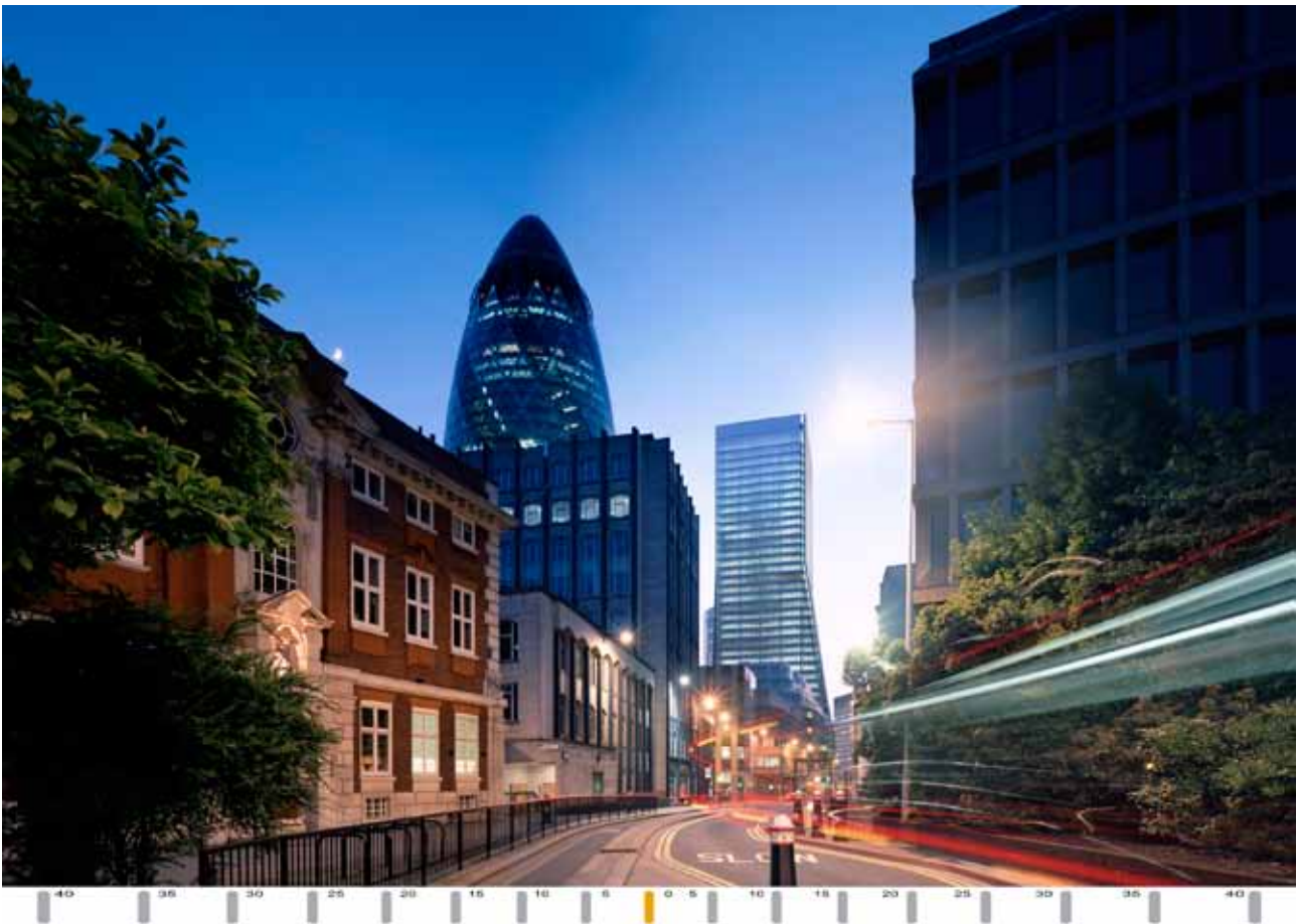
AVR image annotated to show that a wider field of view has been used to include a relevant townscape context. The proposal and the existing tower at 30 St Mary's Axe lie within the central area of the image and thereby avoid obvious distortion
