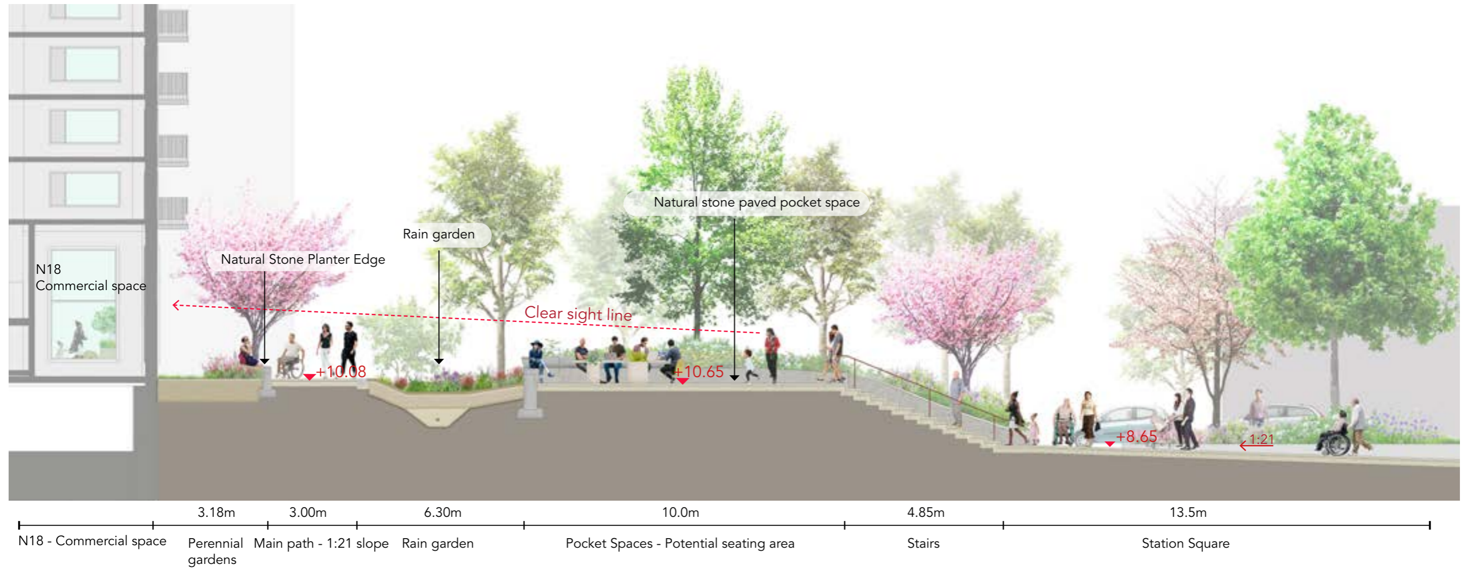
Fig.238 Illustrative section through level change from station square to commercial space inside N18
