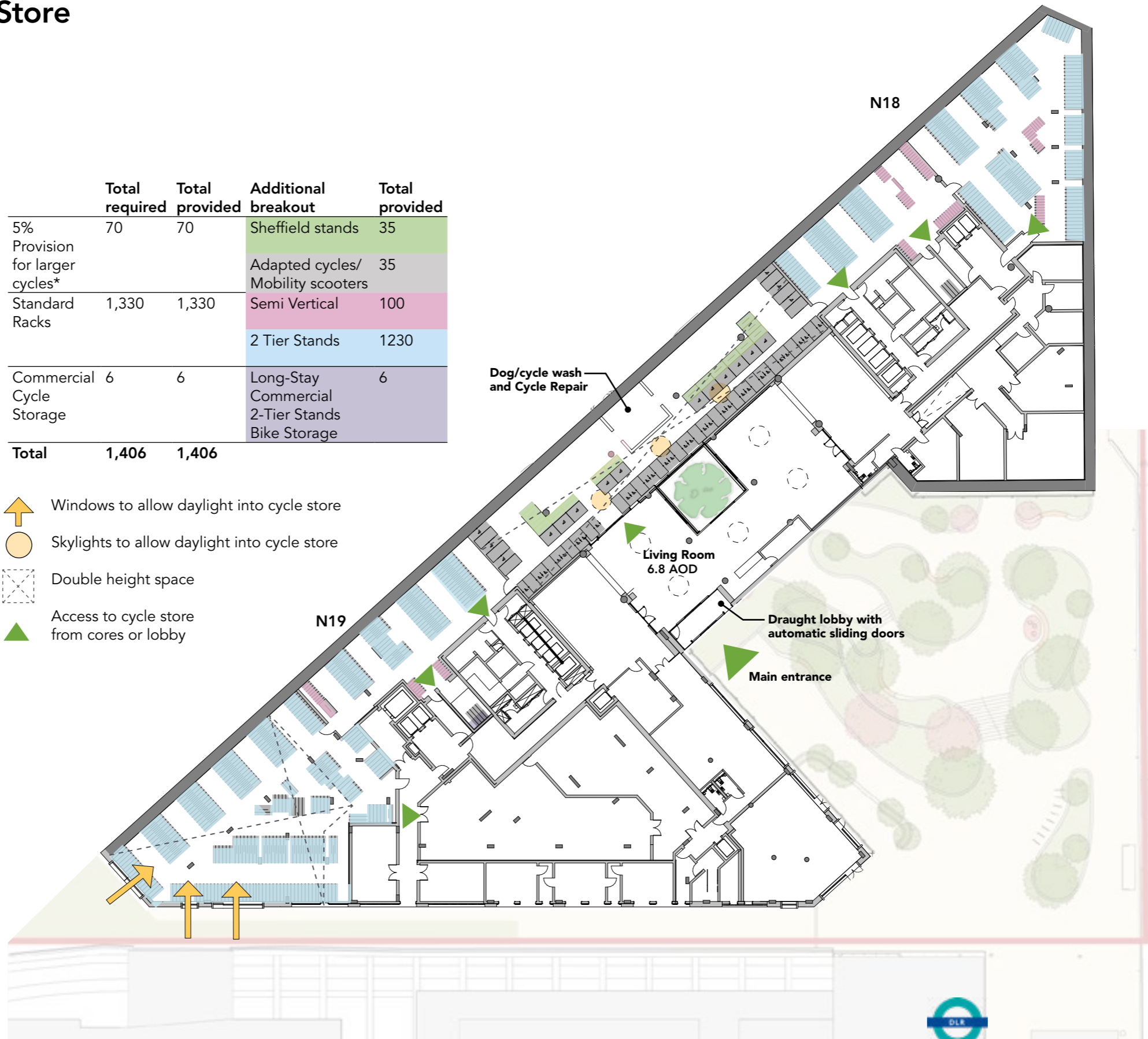
Fig.82 Station Square – Cycle Store
