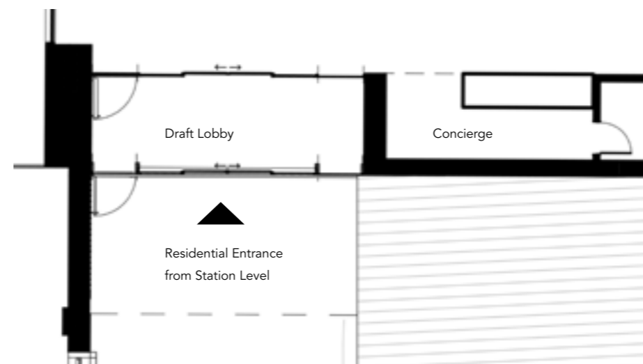
Fig.128 Draught Lobby at Residential Entrance
