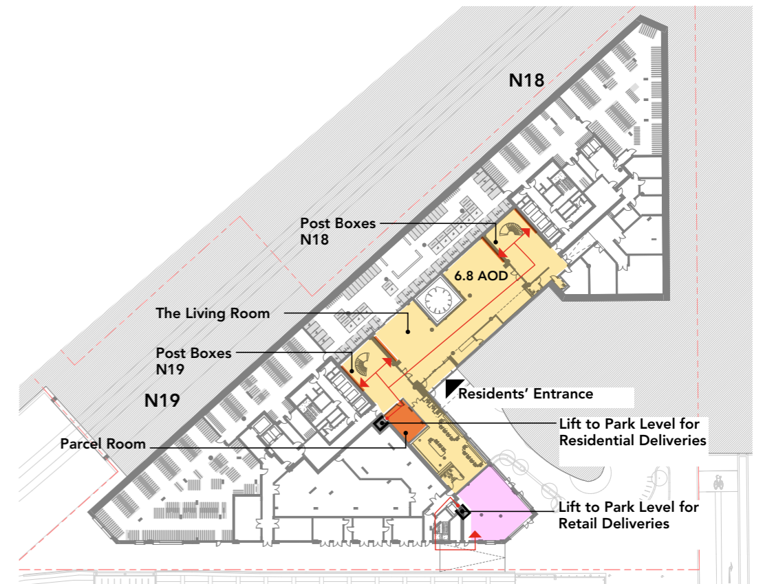
Fig.103 Station Level — Delivery and servicing strategy
