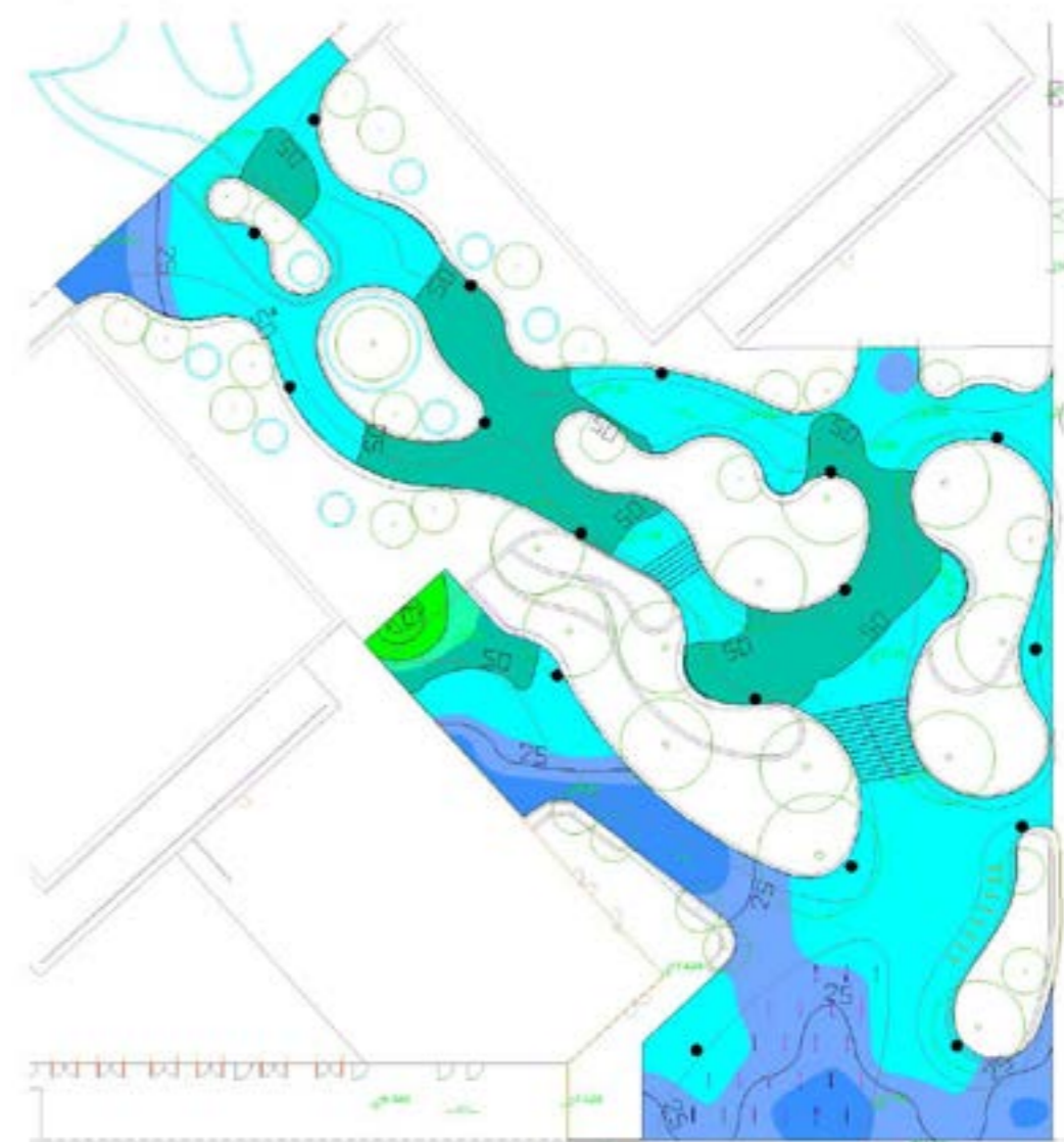
Fig.284 Illustration of lighting calculation result in the public realm between N18/N19 buildings
