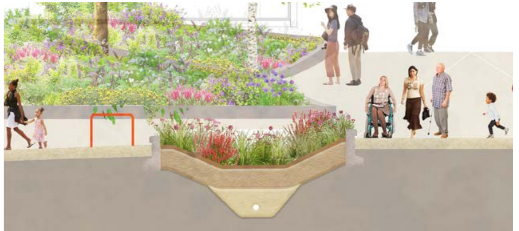
Fig.272 Illustrative section showing proposed rain gardens
