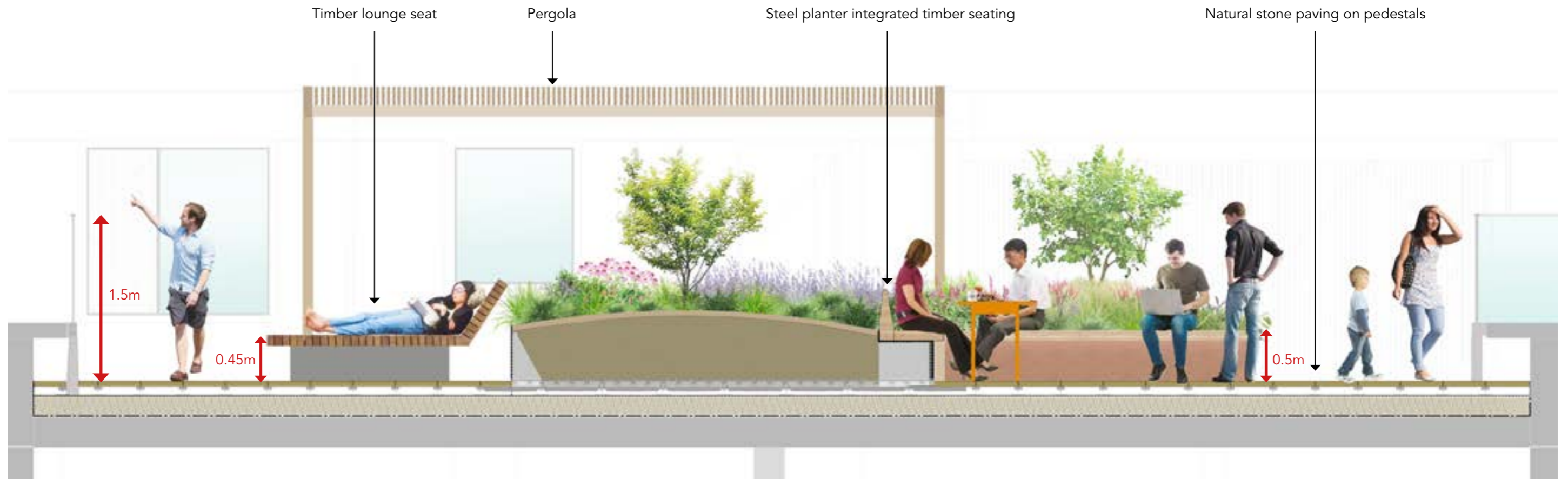
Fig.255 Illustrative section through N19 roof terrace showing the lounge seating and the planter with seating edge
